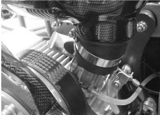
Choke valve shown in "ON" position. Use this position to prime and start the engine initially
