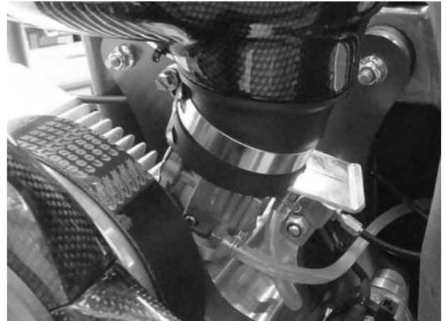
Choke valve shown in "RUN" position. Use this position to run the engine for flying
